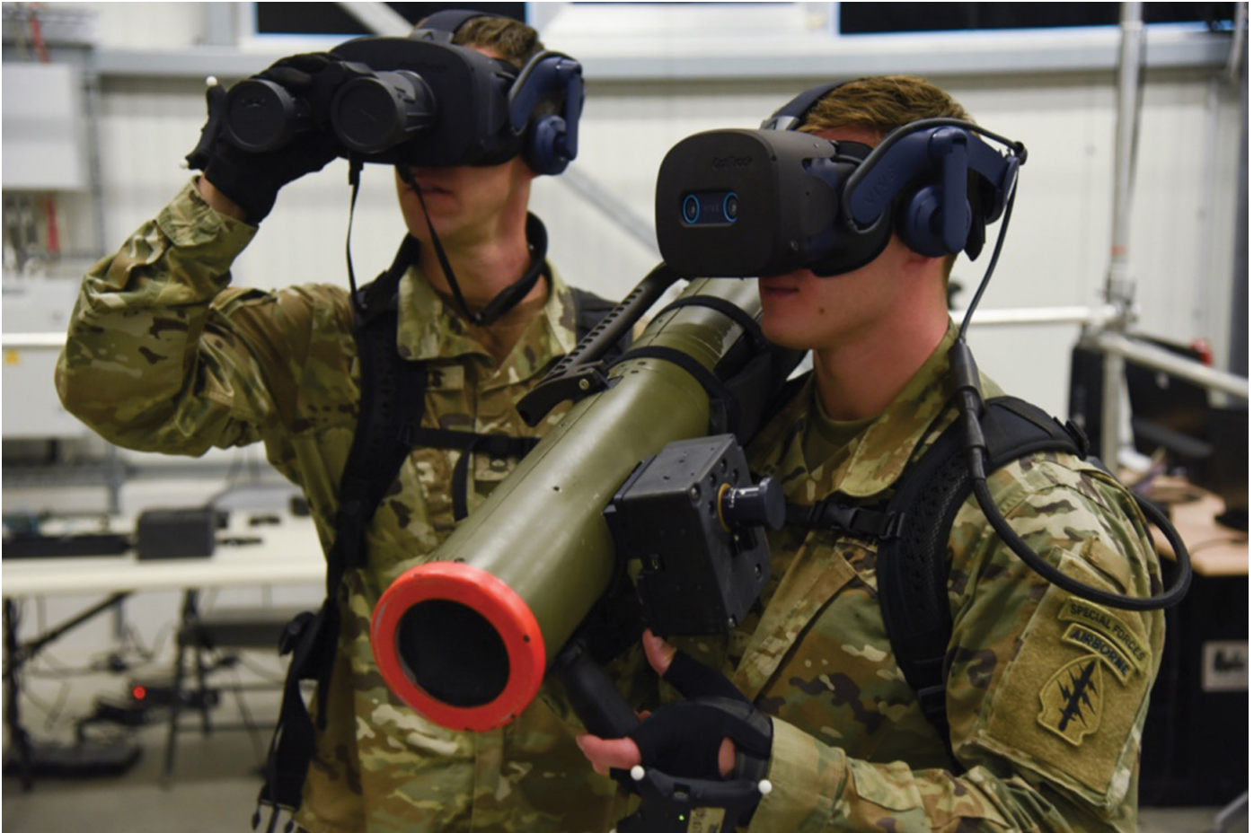
One of the US Army's eight cross-functional teams (CFTs) is dedicated to creating a synthetic training environment (STE) to improve soldier training. Here, US Army soldiers assigned to 10th Special Forces Group (Airborne) use and fire an M3E1 Multi-Role Anti-Armor Anti-Personnel Weapon System (also known as a Carl Gustav recoilless rifle) during a Reconfigurable Virtual Trainer demonstration at the 7th Army Training Command's Grafenwoehr training area, Germany, on February 13, 2020. Source: US Army photo by Markus Rauchenberger. https://www.dvidshub.net/image/6102694/carl-gustav-virtual-training-grafenwoehr
